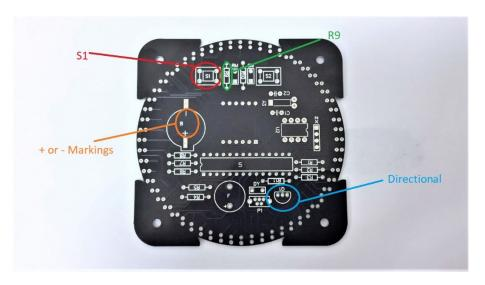
The PCB has component "Identifiers" to help guide with component installation positions. A chart provided below helps identify which component belongs to which position.
